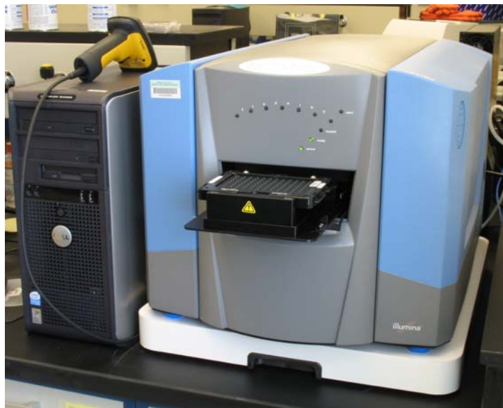
Figure 1. The BeadStation 500GX with an array matrix being loaded for scanning.
